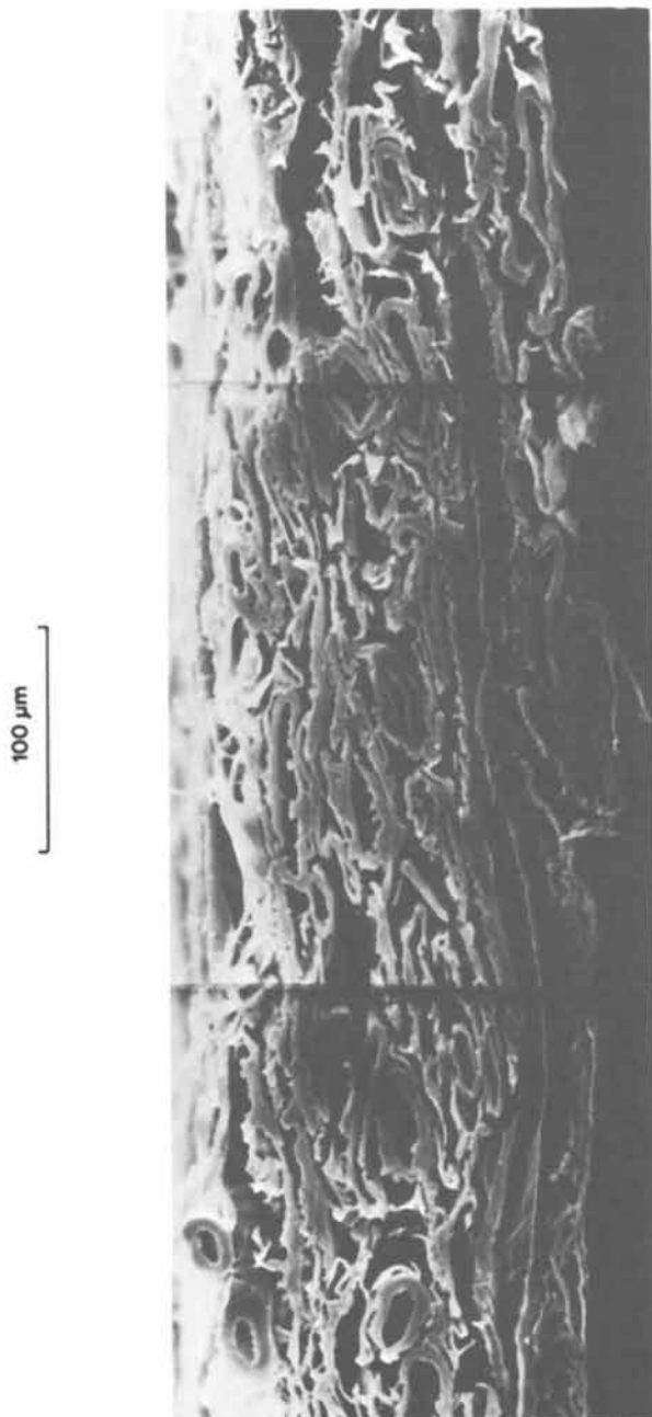
Figure 3. Cross-section microscope picture of a paper sheet showing the preferential orientation of the fibers. (Reproduced, with permission, from Ref. 17. Copyright 1981, American Institute of Physics.)
